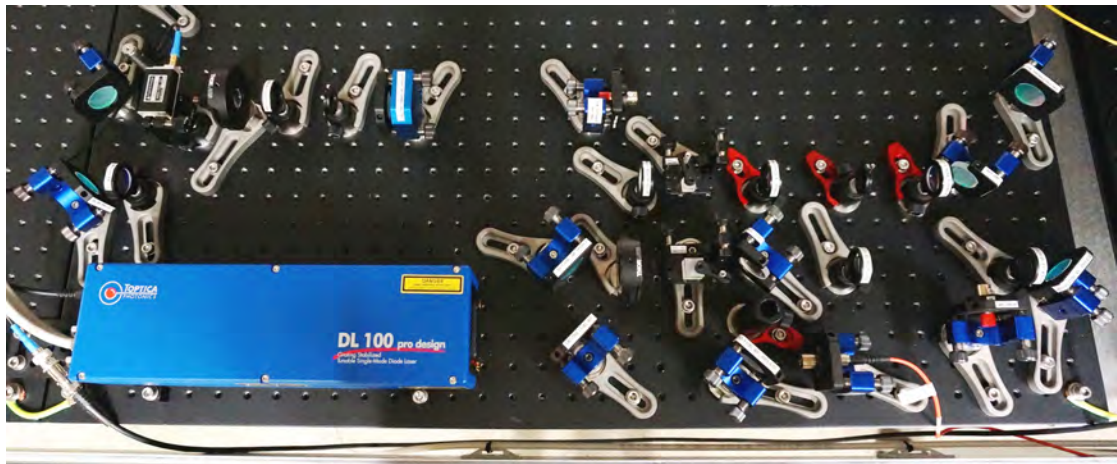
Figure 4.7: Photograph of the 1092 nm laser setup. The configuration follows the schematics in figure 4.6 although for practical reasons the spatial assembly varies to some degree. In the upper left corner one can see the AOM and the optics needed for the double-pass configuration. In the lower right corner two collimators are located leading to the wavemeter (orange fibre) and the ion trap, respectively. The collimator in the upper middle of the picture leads to the cavity. Note that the cavity itself and the PDH setup are not shown in the photograph.
