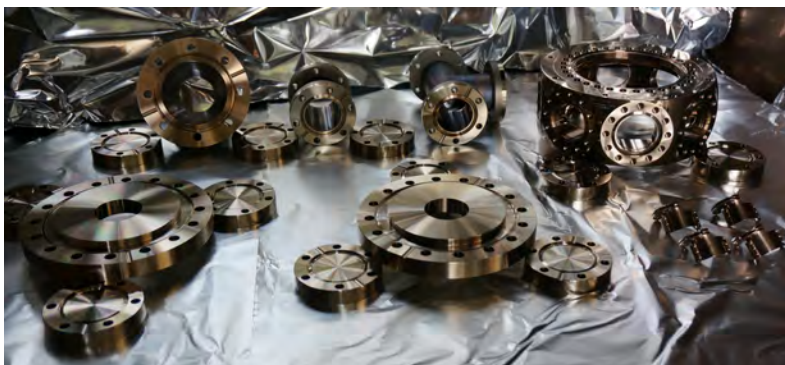
Figure 4.25: Photograph of the parts that were air baked. In the upper right corner one can see the vacuum chamber, in the upper left corner the conical reducer. The two metal plates in the front are the custom-made DN100CF to DN40CF reducers.
