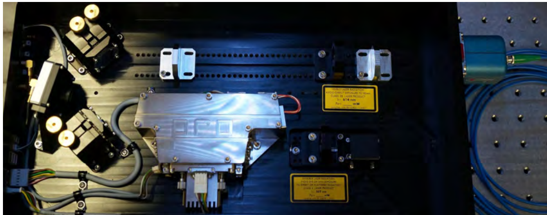
Figure 4.13: Schematic and a photograph of the doubling cavity used for converting the 607 nm – 619 nm light (red line) to the 304 nm – 310 nm UV light (green line). The incoming light is mode-matched with the ring cavity via lenses. The UV light is also beam-shaped before leaving the housing to compensate for astigmatism [33].
