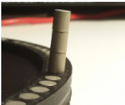
Figure 4.4: Tilted (a) and untilted (b) magnets in one of the magnet holders.
